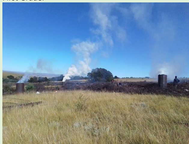
Kilns turning invasive alien black wattle into charcoal, Eastern Cape.
