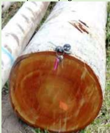
K. senegalensis log from thinning of a 10-year-old, farm forestry stands in coastal lowlands north of Townsville, Queensland Australia. Note the high proportion of dark-coloured wood on the log end (Picture by K. Harding)
